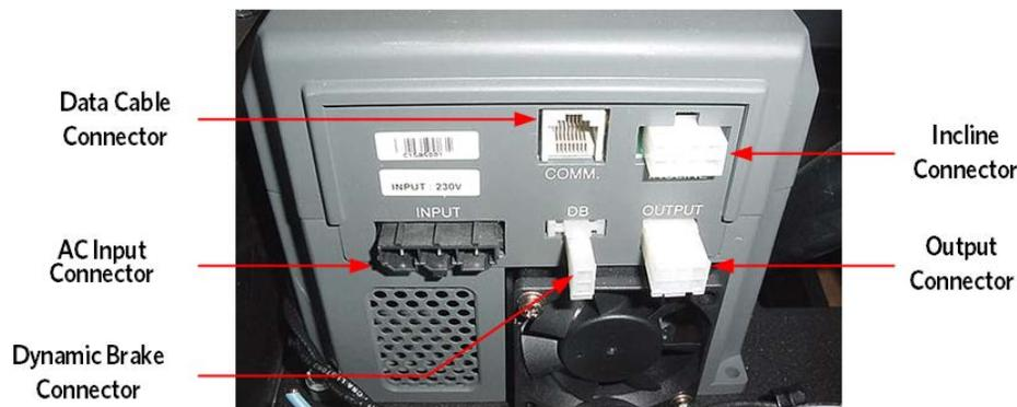
Figure 12: Lower Control Module Connector Numbering
