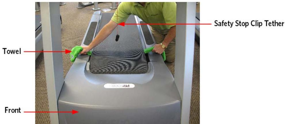
**CAUTION:** If the running belt does not stop, turn off the power using the ON/OFF switch at the front of the treadmill and unplug the power cord. The treadmill must remain out of service until the stop switch is repaired. If the running belt stops, continue with the cleaning procedure
