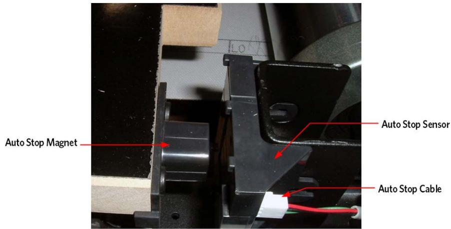
Caution: Do not place the auto stop magnet on or near a steel structure. If the magnet assembly comes in contact with a steel structure and then pulled away from the steel structure, the magnet can become dislodged from the magnet assembly housing. Should this occur, contact PRECOR customer service for possible options for repairing the magnet assembly or to obtain a replacement part.
