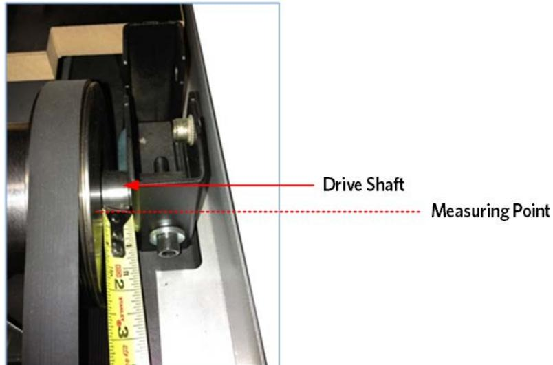
*Figure 42: Measuring Point Frame Cross Beam*
